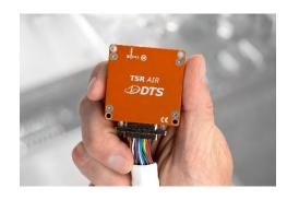
The miniature TSR AIR data logger from DTS includes 11 built-in sensors for shock and vibration testing. The TSR AIR is ideal for automotive, aerospace, and industrial test applications with tight size and weight constraints.
