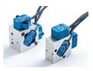
Aluminum mounting blocks make it easy to create a triaxial solution. Additional mounting holes support three Endevco 7264 or MSI 64 accelerometers to create a complete six degrees of freedom package. Two options: ARS PRO Block 21.6 x 21.6 x 10.9 mm (9.9 grams) or the ARS HG Block 21.6 x 21.6 x 16.8 mm (15.2 grams).
