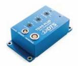
The Level Trigger Device generates a reliable external trigger signal for T=0 for TDAS PRO, TDAS G5, TDAS PLUS or SLICE systems. The crashworthy unit provides two opto-isolated, contact-closure outputs when the user-selected acceleration threshold is exceeded. The isolated output can also be used with any device designed to accept a contact closure (e.g. high-speed imager).
