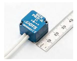
Designed for applications measuring high rates of acceleration and angular velocity, the 6DX PRO-A packages three accelerometers and three angular rate sensors in a compact 19 x 19 x 17.4 mm package.
