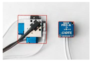
The 6DX PRO-A is 70% SMALLER and 50% LIGHTER than a triaxial block with six individual sensors.
