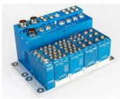
POWER PRO & TDAS PLUS Mini Distributor, shown as part of a complete SLICE PRO solution.
