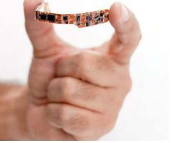
The DDR is a standalone 6-degrees-of-freedom (6DOF) data logger that measures linear and angular acceleration. The ultra-light logger is designed to monitor short duration events in small devices under test.
