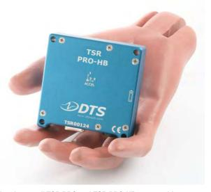
The ultra-small TSR PRO and TSR PRO-HB are portable data loggers with built-in triaxial accelerometers. Ideal for both short duration tests and long term monitoring, the TSR time and date stamps each event and stores up to 2,000 events in flash memory.
