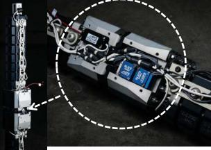
The FLEX PLI Leg supports up to 48 channels of integrated SLICE NANO data acquisition. Embedding the data recorders eliminates trailing cables that may get tangled or cause issues with noise or data loss. The turn-key solution is engineered to maintain proper mass, center of gravity (CG) and moments.
